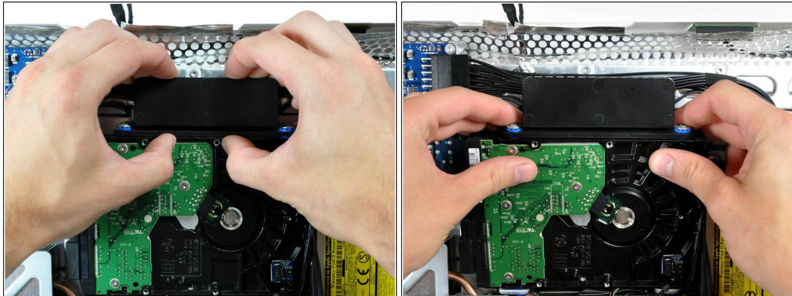
**⚠** Pressing the top of the hard drive bracket down to release it from the rear case requires a substantial amount of force, so we recommend laying your iMac stand-side down on a table to avoid knocking it over.
